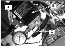
**Safety Valve (C):** If the pressure switch does not shut off the air compressor at its "cut-out" pressure setting, the safety valve will protect against high pressure by "popping out" at its factory set pressure (slightly higher than the pressure switch "cut-out" setting).
